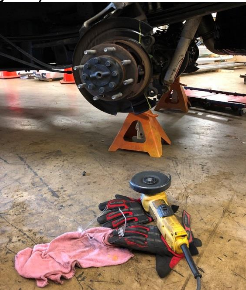
Photo 5: Use the proper safety equipment when cutting backing plate (safety glasses as well work gloves)
