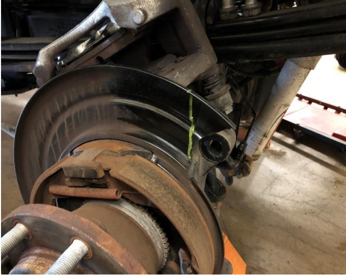
Photo 4: Lower cut line on backing plate
