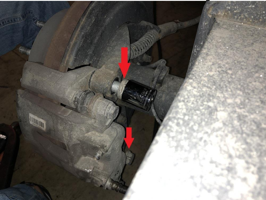
Photo 2: Cradle bracket bolts that are to be reused during install of new caliper
