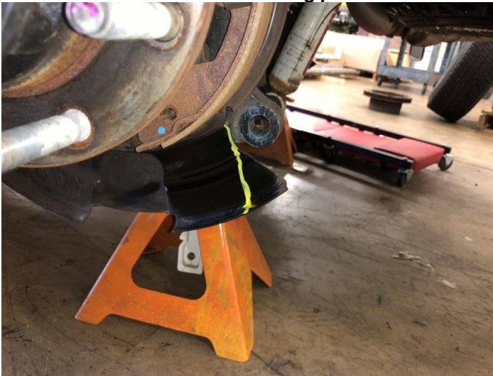
Photo 5: Use the proper safety equipment when cutting backing plate (safety glasses as well work gloves)
