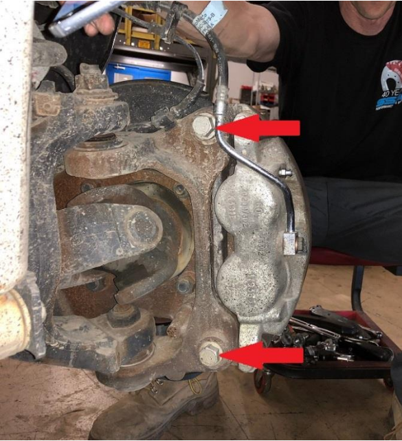
Photo 6: Cradle bracket bolts that will be reused during install
