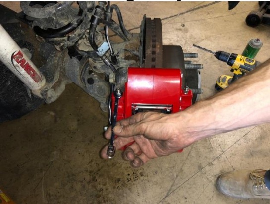
Photo 7: Bleeding the system
