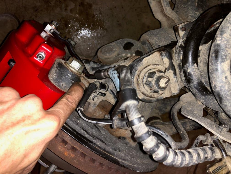
Photo 5: Ensure line does not make contact with bolt or knuckle after bend is made in line
