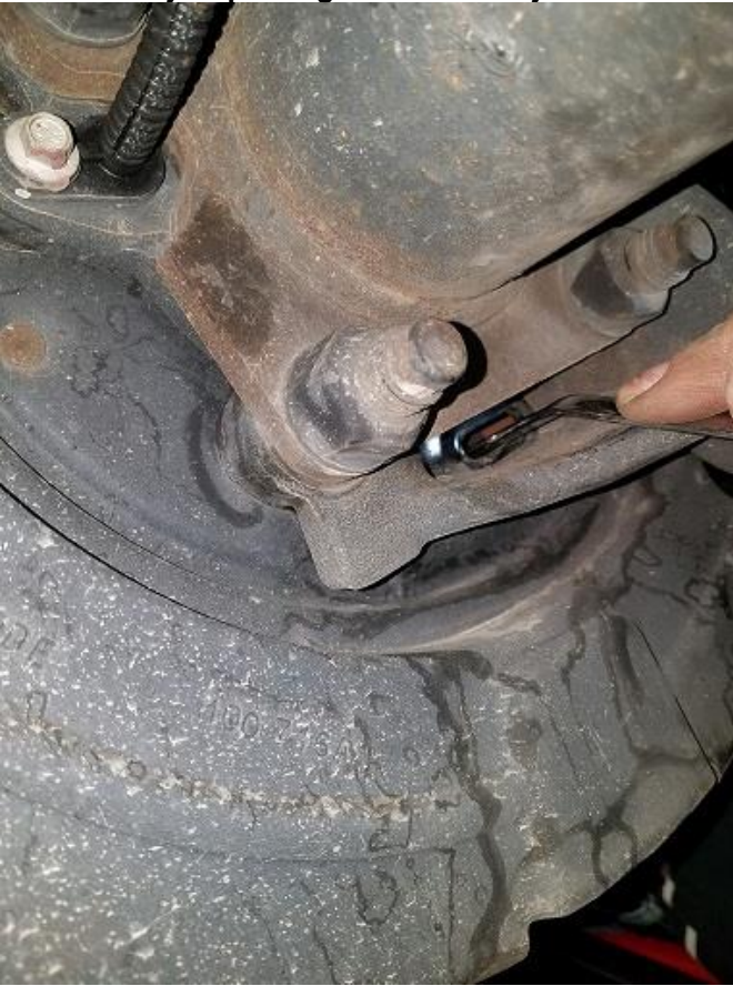
Photo 2: Cradle bracket bolts that are to be reused during install of new caliper
