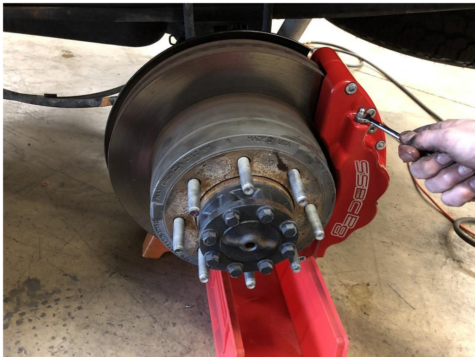
Photo 3: Bleeding the system, make sure to bleed both bleeders starting with the outside bleeder, as shown in the picture below.
