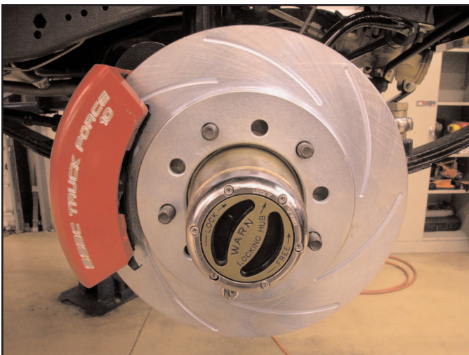
Photo 5: Slide caliper over rotor and torque slider bolts to 40 ft/lbs
