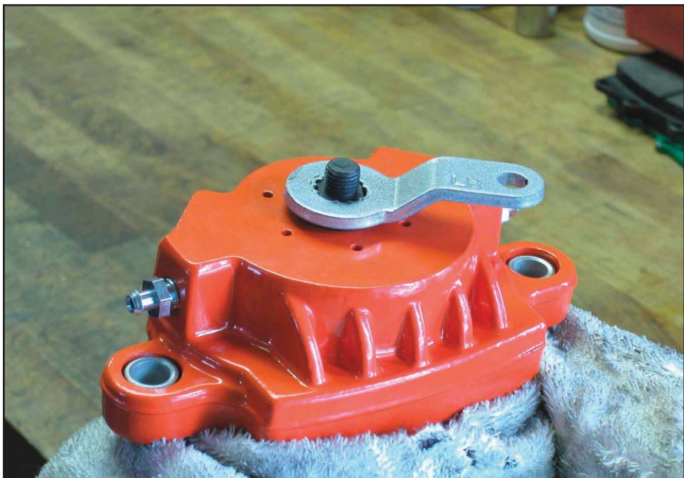
Photo 4: The parking brake lever can now be removed from the stud. Rocking the lever up and down will help free the lever from the stud.
