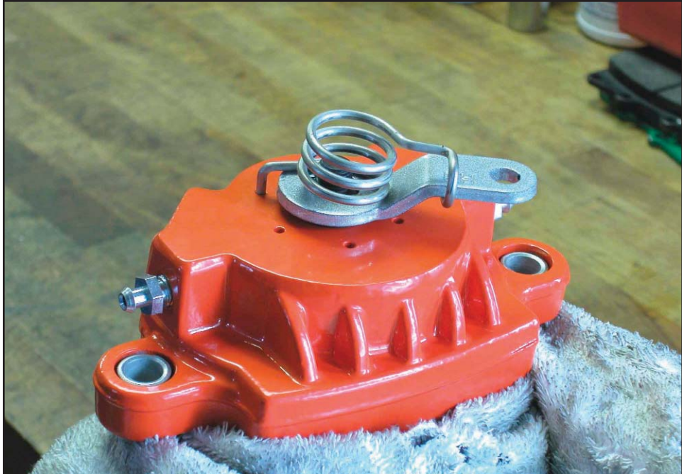
Photo 3: With the retaining nut removed, the parking brake return spring can be removed. Notice how the spring fits with the loop hooked onto the parking lever and the straight end pushed into the hole on the back of the caliper.
