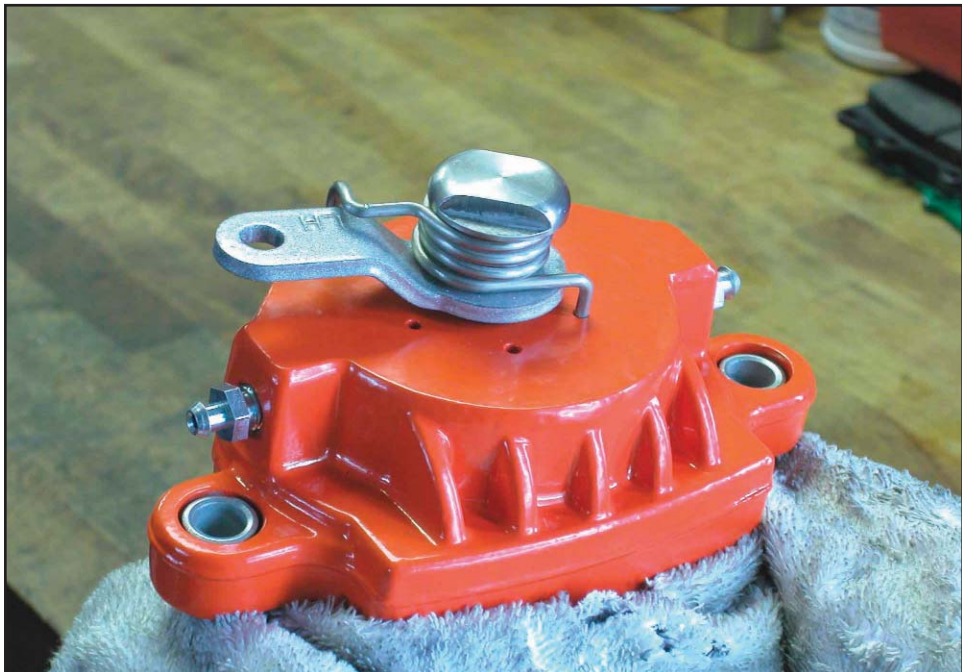
Photo 8: The caliper is now ready for installation.
