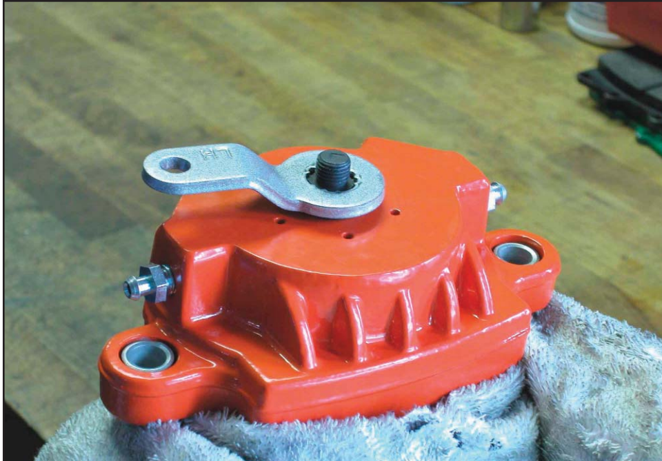
Photo 5: Install the lever in the new position, making sure the notches in the lever align with the hex shoulder of the stud. This insures the lever will turn the stud and not simply spin without engaging the parking brake.
