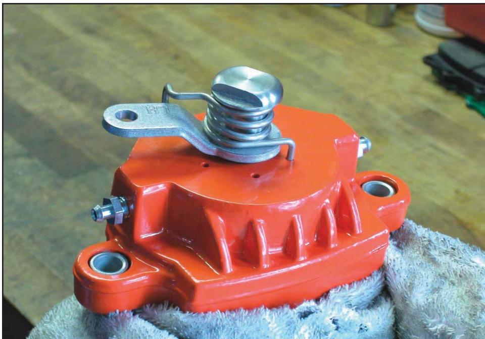
Photo 6: Reinstall the spring and retaining nut. Be sure to install the straight end of the spring into a hole in the back of the caliper; this will create spring tension as soon as the lever is moved.
