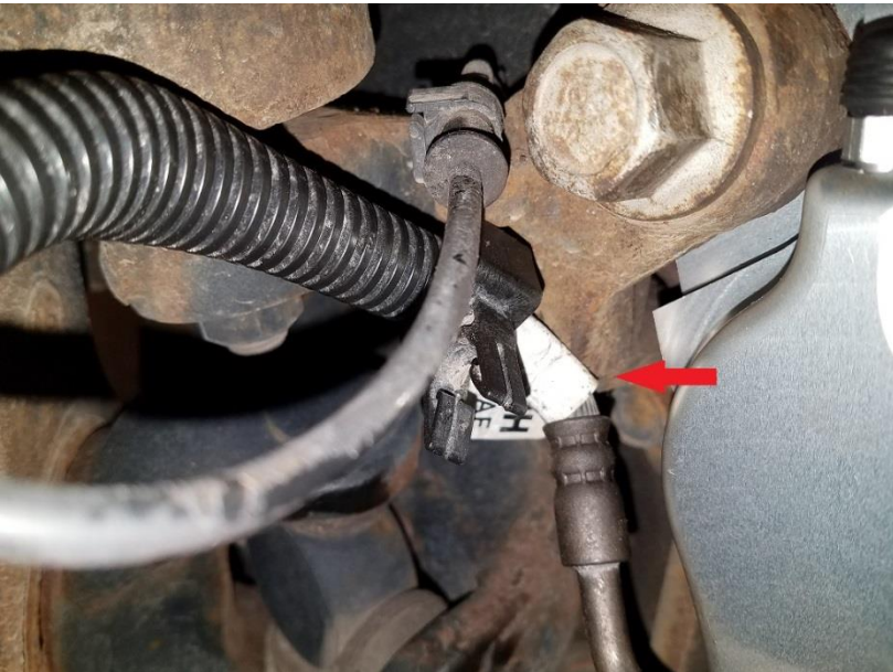
Photo 2: Bend hard line to make sure flex hose is not rubbing where indicated
