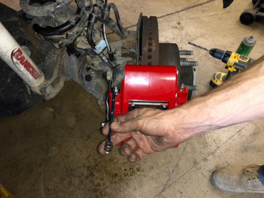
Photo 3: Bleeding the system
