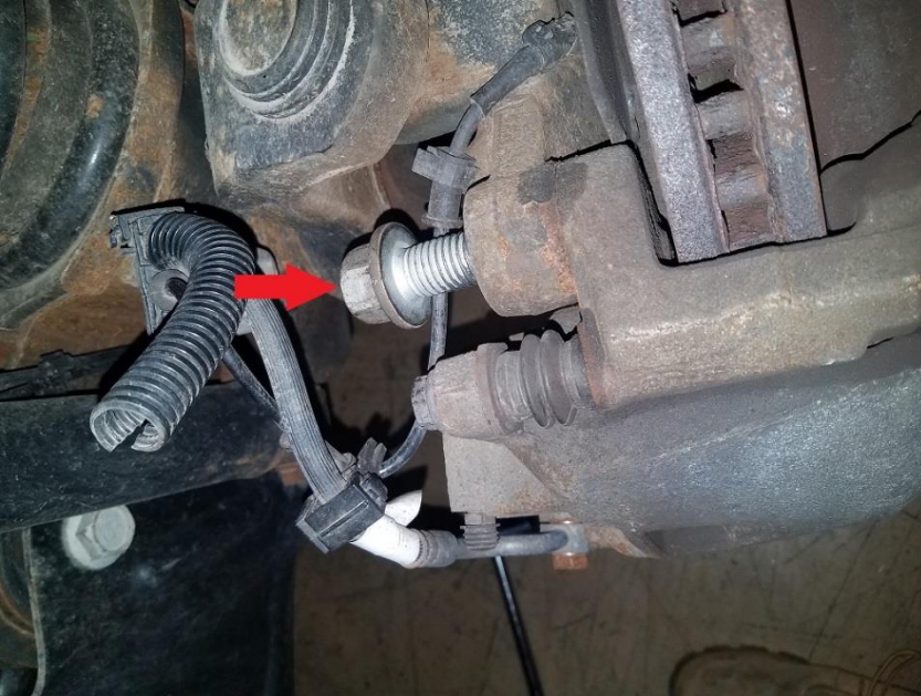
Photo 1: Cradle bracket bolts that will be reused during install
