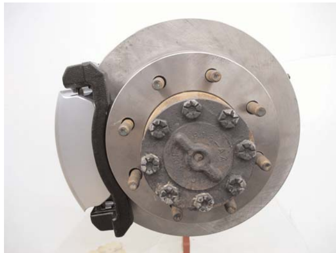
Slide the caliper assembly over the rotor and secure with the original bolts. Torque to 125 ft/lbs.
