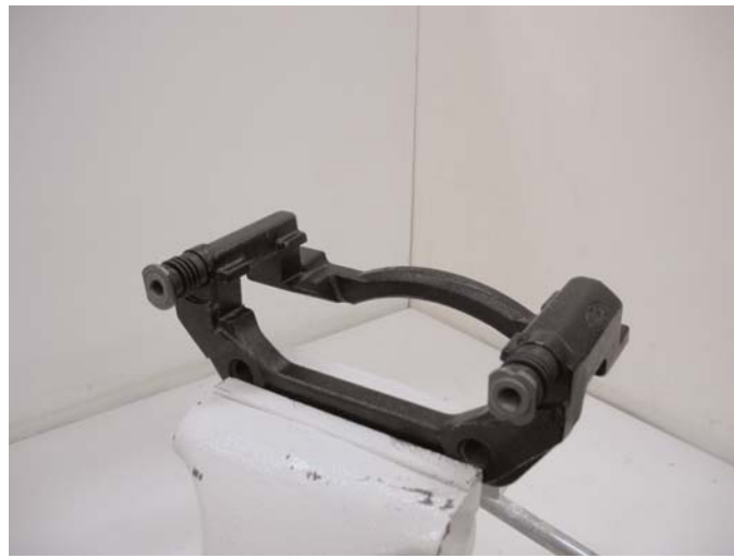
Install the supplied dust boots on the cradle. Lubricate the original slider bolts with a high temperature grease and install in the cradle.
