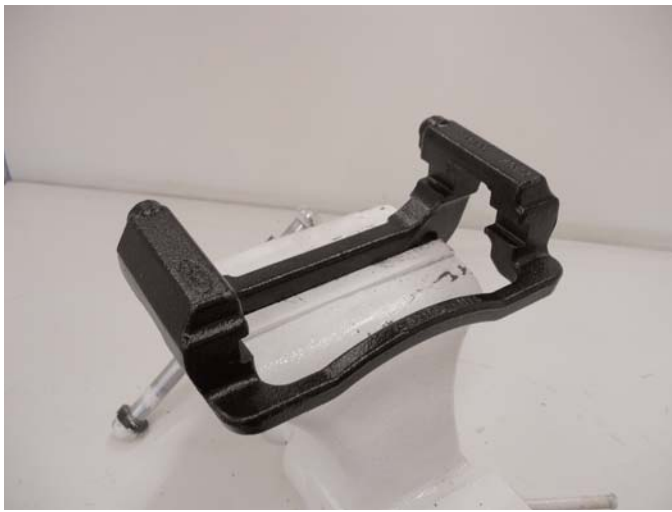
Photo of factory cradle bracket with all of the hardware removed. The cradle can be left on the truck if the rotors are not being replaced.
