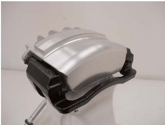
Install the caliper on the assembly and secure with the original hex bolts. Torque to 25 ft/lbs.
