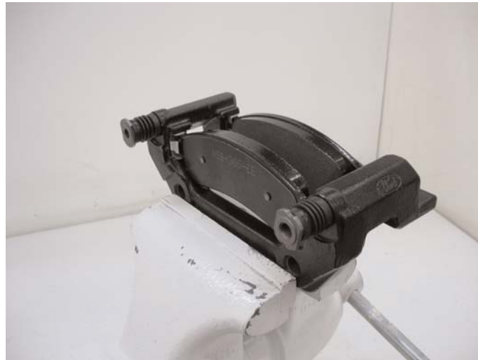
Install the pads in the cradle with the friction material facing in.
