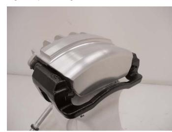
Install the caliper on the assembly and secure with the supplied M8 hex bolts. Torque to 25 ft/lbs.
