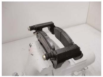
Install the pad clips on the pads and install in the bracket.
