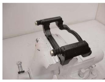
Install the supplied dust boots and slider bolts in the cradle. Lubricate the slider bolts with a high temperature grease.
