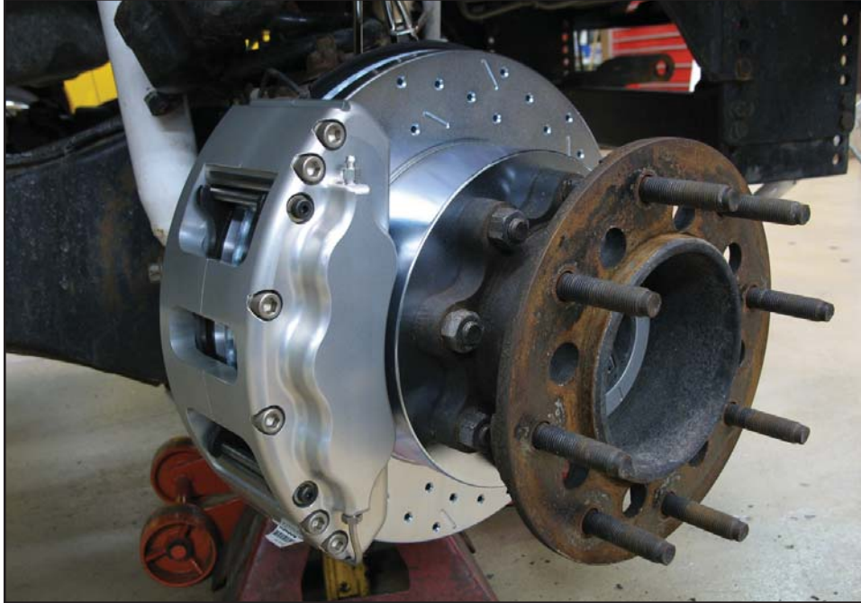
Complete installation of Quick Change calipers
