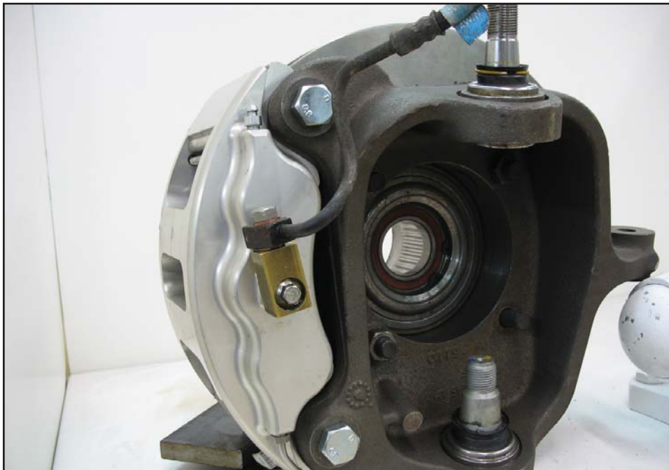
Proper connection of adapter block and flexline.
