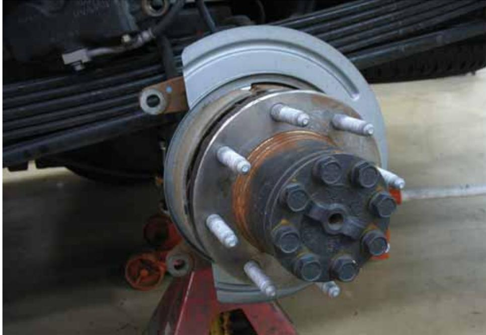
If replacing rotors also, slide the brake rotors off the hub
