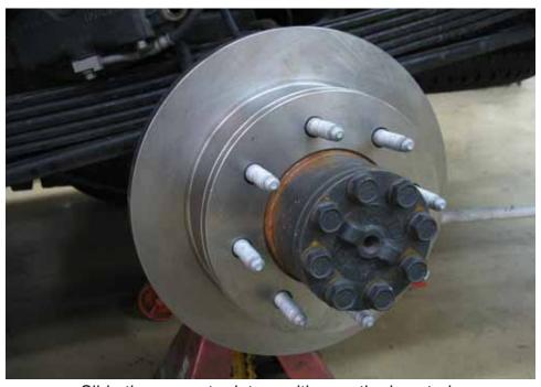
Slide the new rotor into position on the lug studs
