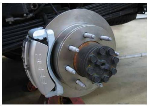
Slide the new caliper assembly over the rotor and secure with the 14mm bolts removed earlier. Torque to 125 ft/lbs.
