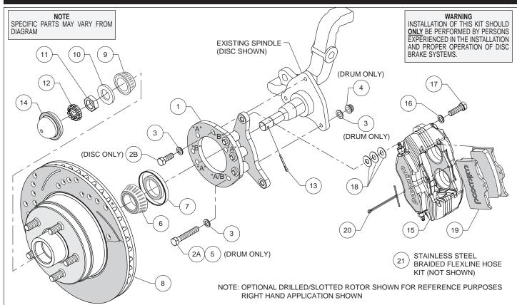
Figure 4. Typical Installation Configuration
