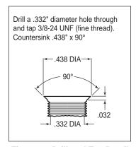
Figure 2. Drill and Tap Detail
