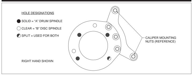
Figure 1. Wilwood Caliper Mounting Bracket
