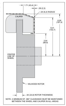
Figure 3. Wheel Clearance Diagram
